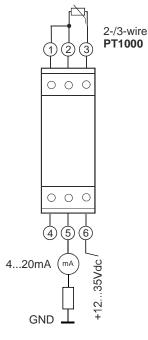
The output current follows linear at the input
