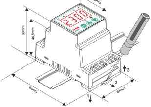
For mounting the device to the panel; Push the device in direction 1, the rails provide the key to keeping the rail.
